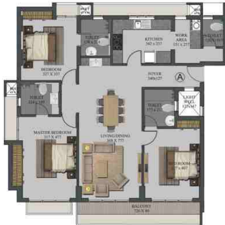
UNIT A (3 BHK) 10TH - 11TH FLOORS AREA : 1762 SQFT (163.79 SQM) DECK AREA : 139 SQFT
